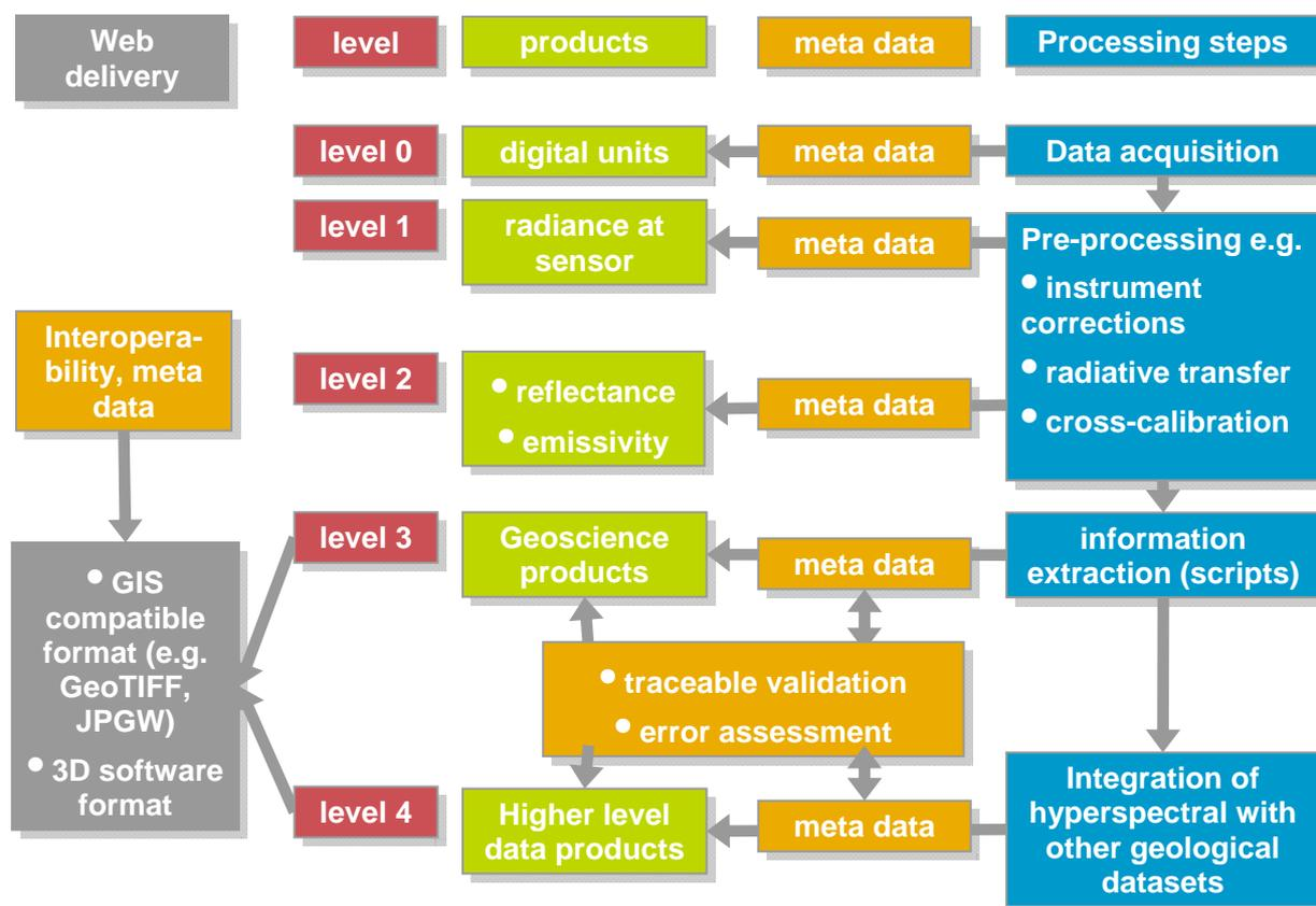
Figure 1. Strategy for processing of hyperspectral data
